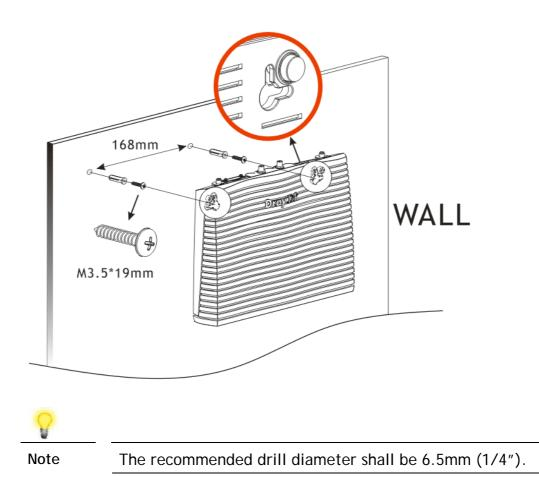
3. When you finished about procedure, the router has been mounted on the wall firmly.
